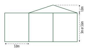
An example of a side profile of a standard pitched roof cricket net facility and heights as specified in AS1725.4 - 2010.
