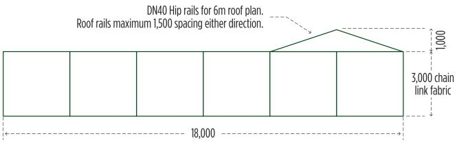
Typical two pitch cricket net fencing enclosure Type B with pitched roof design.
